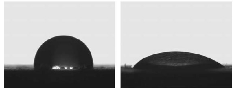
Fig. 9. Application for the DBD plasma jet: surface modification of wood (left: waterdroplet on untreated wood, right: waterdroplet after the plasma jet treatment).
