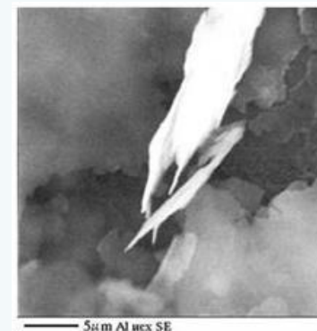
Al(N4), ( S=2.7 \text{ m}^2/\text{g} ) \langle L \rangle \sim 0.5 * 21,3 \mu\text{m}
